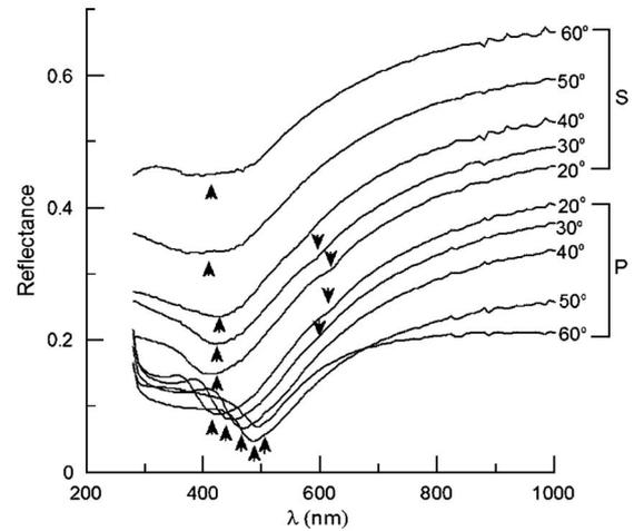
FIG. 3. Measured optical reflectance spectra of 60 nm thick nanocorrugated Co film (particle size of initial PMMA colloidal crystal is 290 nm) for s- and p-polarization of the incident light and for different incident angles. Up arrows indicate minima due to localized dipole mode; down arrows indicate remnant minima due to propagative surface plasmon mode.
