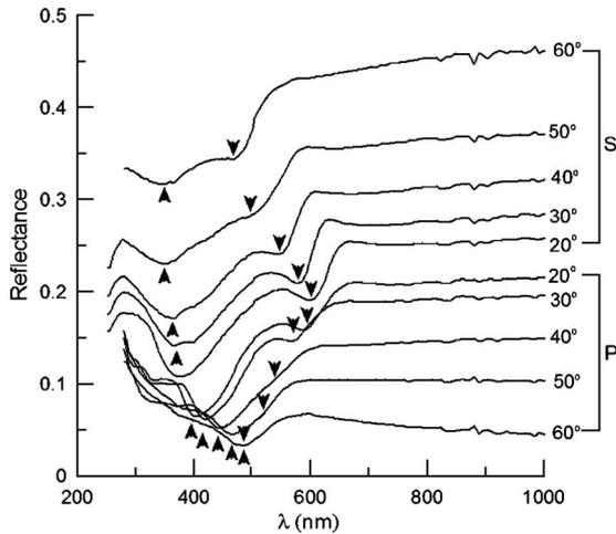
FIG. 2. Measured optical reflectance spectra of 30 nm thick nanocorrugated Co film (particle size of initial PMMA colloidal crystal is 290 nm) for s- and p-polarization of the incident light and for different angles of the light incidence. Down arrows indicate minima due to propagative surface plasmon mode; up arrows indicate minima due to localized dipole modes.
