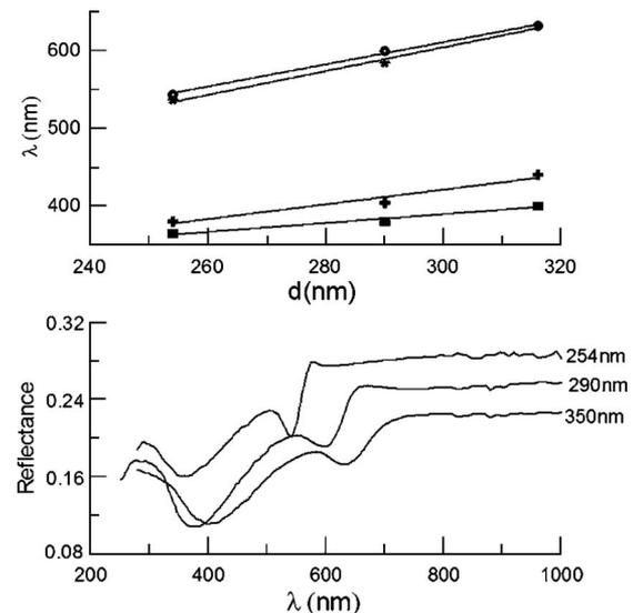
FIG. 4. Scaling of the reflectance spectrum of nanocorrugated films with the diameter of the particles of the colloidal crystal. Upper graph is the positions of lw and sw reflectance minima for the samples with different diameters (Co thickness is 30 nm) for the incident angle 20°: Circles and squares—s-polarization, stars and crosses—p-polarization. The bottom graph is the reflectance spectra for s-polarized light with the angle of incidence 20°.
