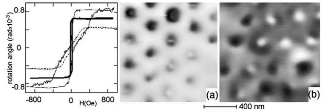
FIG. 5. Magnetization curves of the nanocorrugated Co films (thin line for 30 nm film, dashed line for 60 nm film), PMMA particle diameter 290 nm. Thick line is a magnetization curve of the flat 30 nm Co film. (a) MFM image of the 30 nm sample at  $H=0$ , magnetization states of Co hemispheres looks like magnetic vortex. (b) MFM image of the 60 nm sample, both vortices and single domain states are visible.
