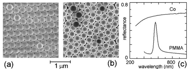
FIG. 1. SEM images of the PMMA colloidal crystal: (a) before deposition of the Co film, (b) after deposition of the film. The single particles are seen on the surface in both cases. (c) Reflection coefficient of the initial PMMA colloidal crystal (particle size 290 nm) and reflection coefficient of the control Co film (thickness 30 nm) for 45° of incident angle for s-polarizations.
