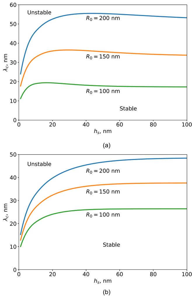
FIG. 4. The skymion stability diagram for the various (a) dot and (b) anti-dot radii. The thickness of the ferromagnetic film is (a)  $h_f = 1.5$  nm and (b)  $h_f = 10$  nm.
